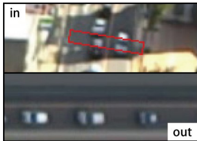
Time-lapse conversion in: narrow line in video out: time-lapse image
